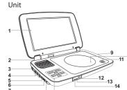
LCD screen HDMI jack **DC IN 9V - 12V** jack AUDIO / VIDEO OUT iack CHARGE / STANDBY / ON switch VOLUME control
